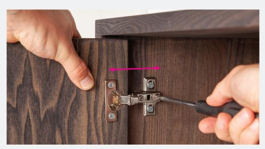
2: Then gently pull/push the door in the desired direction and tighten the screw again. Repeat the process on all hinges if necessary. Then close the door and check if the distance is as desired - repeat the adjustment until the desired result is achieved.
