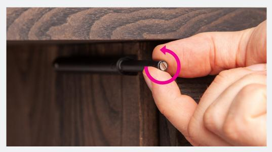
3: On the opposite side of the door, the adjustment pin can also be adjusted in or out on the push mechanism to achieve the desired result.
