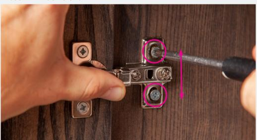
By loosening the screws on <u>all the door hinges</u>, the doors can be adjusted up and down by moving the fitting into the free space. When the desired position is achieved, tighten the screws again.
