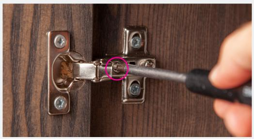
With this screw, the width of the doors can be adjusted. Close the door and check if the distance fits - repeat the adjustment until the desired result is achieved.
