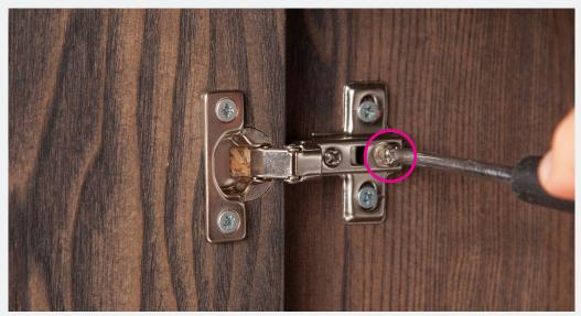
**1:** With this screw, the doors can be adjusted in depth on the hinge side both above and below. Start by slightly loosening the marked screw.
