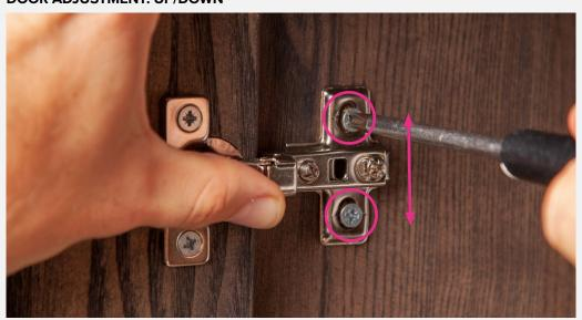
By loosening the screws <u>on all the hinges of the door</u>, these can be adjusted up and down by pushing the bracket in the clearance. Once the desired location is achieved hold the door and tighten the screws again.
