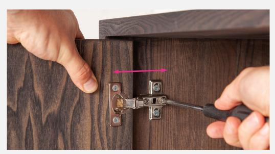
**2:** Gently push/slide the door in the desired direction and tighten the screw again. Repeat the process on all hinges if necessary. Then close the door and check if the distance is as desired repeat the adjustment until the desired result is achieved.
