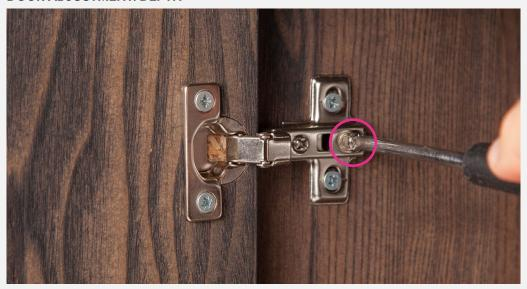
**1:** With this screw, the depth of the doors can be adjusted in the hinge side, both in the top and bottom. Start by loosening the marked screw slightly.
